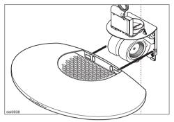
Hang the canopy from the motor assembly by placing the holes at the rear over the hooks on the lower edge of the assembly. Be careful not to pinch any wires.
